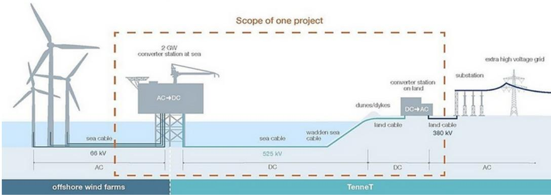
The proposed TenneT 2GW HVDC grid model standardizes the layout for onshore/offshore HVDC substations. This system informs the recommended HVDC system design.
