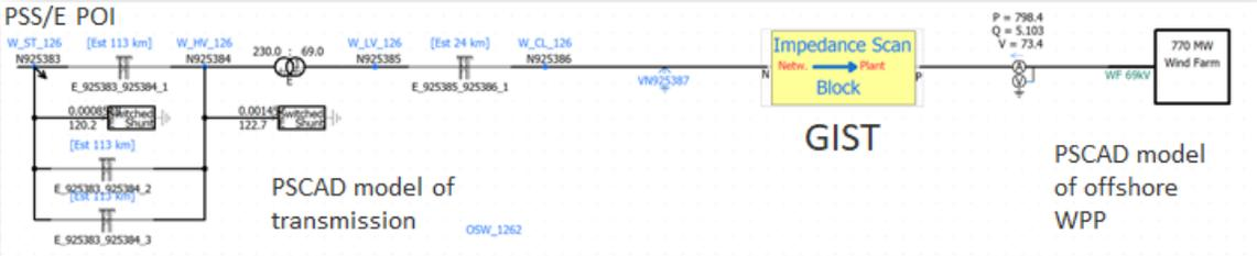
Figure 43. GIST used between PSCAD model of an offshore WPP and PSS/E model of the grid
